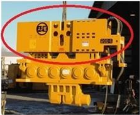
APE Vibration Suppressor and vibro bolted together as ONE Complete Unit
